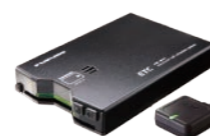
Automotive ETC (Electronic Toll Collection) System Enable toll payment processing on toll roads without the need for halting the vehicle at tollgates.
