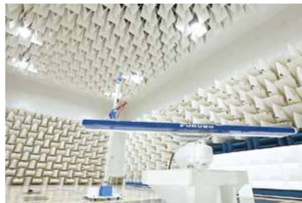
EMC testing of a radar antenna
