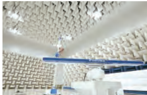
EMC testing of a radar antenna
