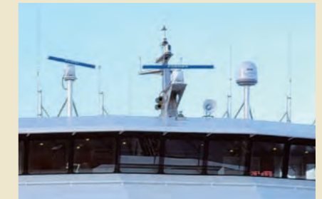
FURUNO radars installed on Seastreak's Courageous ferry
