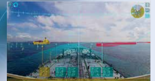
Display image of the AR Navigation System. Azimuth, AIS, own ship position, ship speed, and other information such as the route and waypoints are superimposed over the live video imagery.
