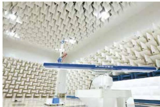
EMC testing of a radar antenna
