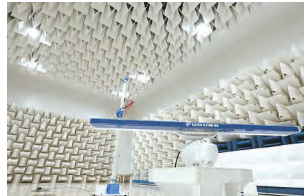
EMC testing of a radar antenna
