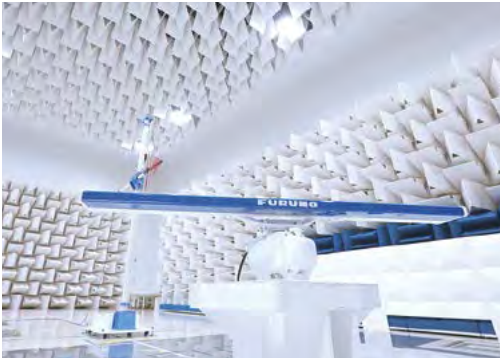
In-house EMC* testing environment
