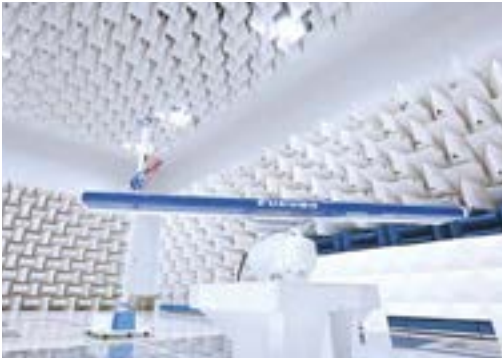
In-house EMC* testing environment
