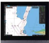
ECDIS (Electronic Chart Display and Information System)
